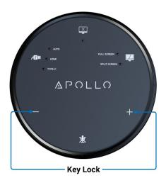
If Apollo becomes inaccessible on the network and a factory reset cannot be performed via the web interface, you can also press and hold the **mic mute** and **video mute** buttons together for at least 5 seconds. This will perform a hard reset and default all settings to factory.
