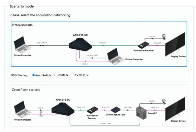
**Note**: In 'Zoom Room' scenario mode DisplayLink is not supported, only USB-C or HDMI connections can be used.
